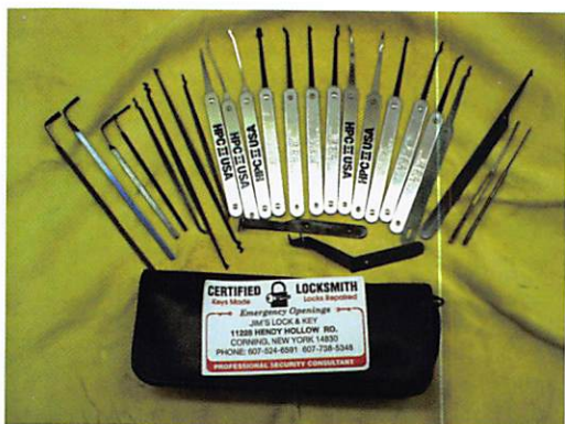
Jim Rouse also relies strictly on HPC. Note the wide variety of key extractors and a few double-ended picks.
