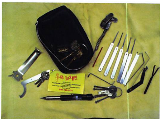
Carl Orozoco's pick set contains a plug spinner, a single Rytan pick, a host of HPC and a variety of extractors and tension wrenches.
