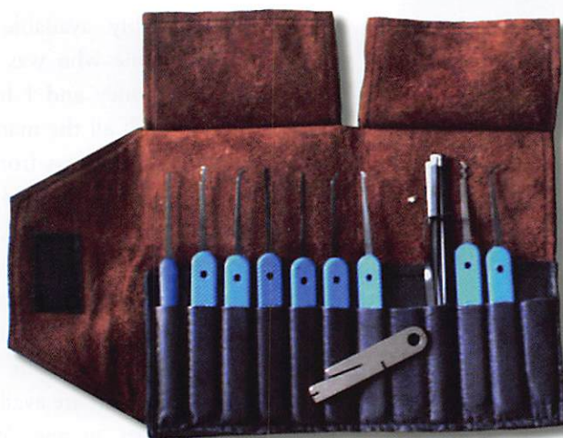
A nice assortment of Peterson picks, with the tool for bending your own tension wrenches in plain view. I was very impressed with the quality of this set.
