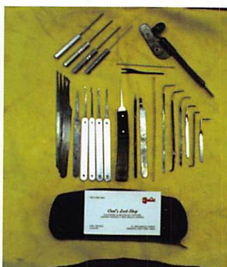
Mark Fuller, CPL, (one of my esteemed employers,) carries a plug spinner, some extractors, a combination of HPC and Rytan, and a knitting needle in his pick set!
